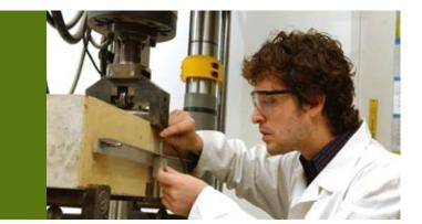
Preparing for a bending test on steel fiber-reinforced concrete
