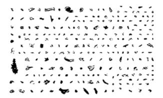
This is a close-up of particulate material in hydraulic fluid from a glass fiber filter. The smallest particle is 20µm while aircraft hydraulic systems require absolute filter ratings of 5µm. *ref: US AED*
